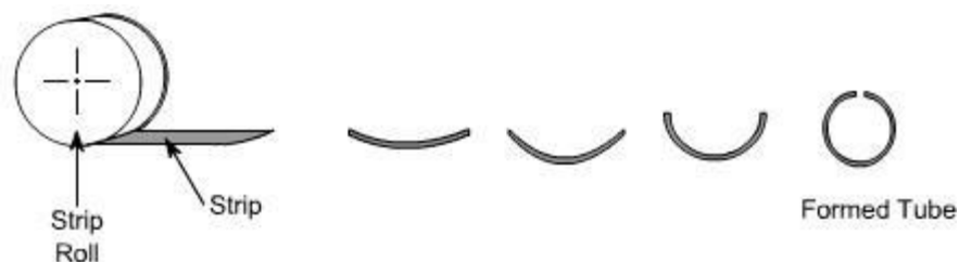
Fig 11.10: Forming of Tube from Strip
